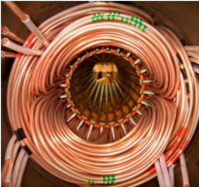
Motors for special applications with PE2/PA insulated winding wires
