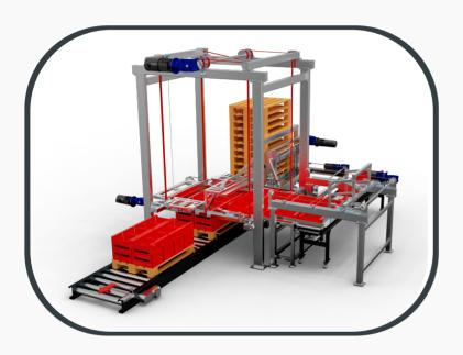
After the process of sorting and weighing the boxes/cartons is completed, the packaging goes to the palletizer. The method of creating pallets is programmable by the user and is adapted to various packages of different dimensions.
