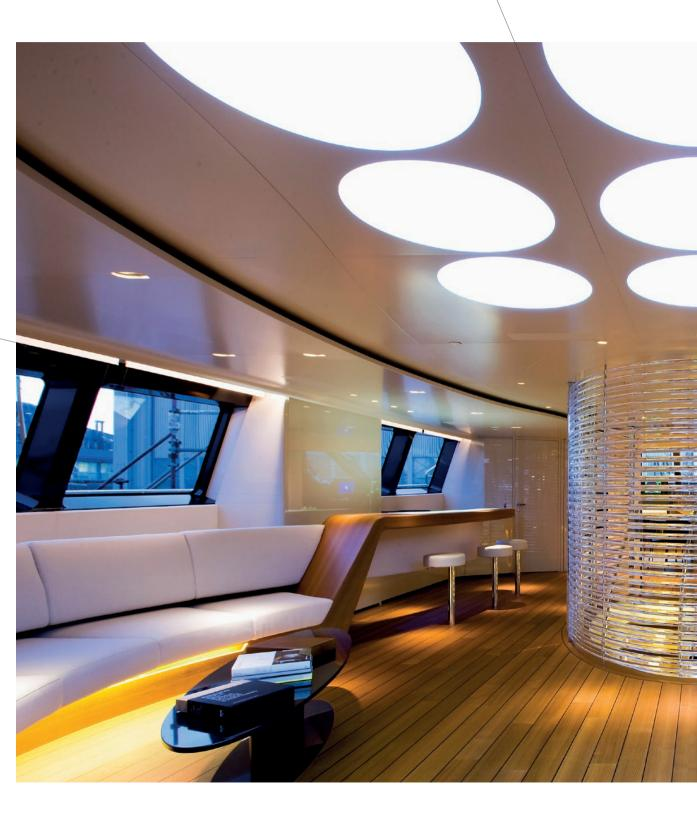
Backlit ceiling in Corian<sup>®</sup>. The light, as a real pure element, appears as visible circles passing through the ceiling itself, due to its translucency. You can see the light but you don't see the light source.
