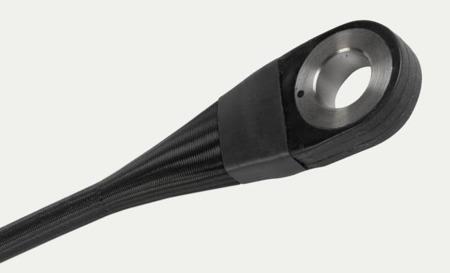
**Future Fibres** pioneered this low weight standing rigging solution in 2001. Utilising an unidirectional wound fibre core, **Fibrelite** rigging is the next step in the evolution of rod rigging. It represents the first step of the movement towards achieving weight savings in rigging by using fibre rigging over nitronic rod.
