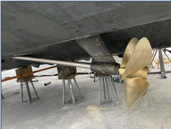
Montecarlo Yachts 105ft – Shaft lines overhaul
