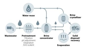
One way of reducing energy consumption is to reduce the amount of water that needs to be evaporated by changing from a thermal to a membrane-based process. This is supported by studies that show an efficiency gain of up to 75% when going from the thermal-based to the membrane-based process.
