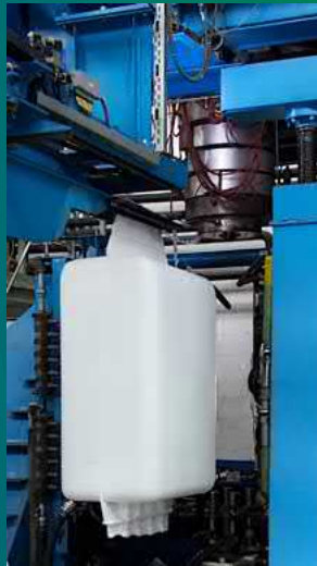
Blow molding system
