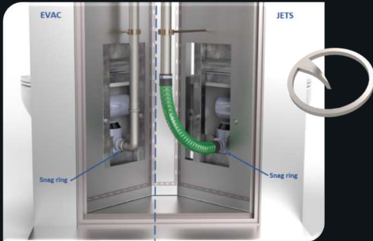
Typical BW pipe layout
