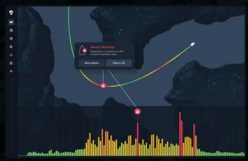
Upcoming feature for collision and grounding warnings and alerts, notifying operator or observer if vessel has an impact with a physical object.
