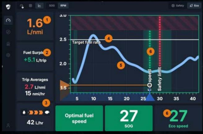
**IMAS®** Helm Eco Speed, can optimize fuel use or available range, dynamically predicting a prevailing fuel curve, speed & RPM, continuously adapting to each vessel and conditions & continuously improving.
