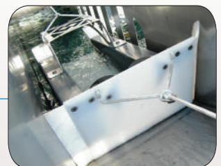
Self-adjusting grease scraper with limited water removal
