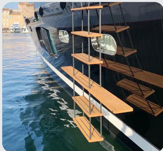
Pilot ladder hangs in mid-air with no firm support against the hull
