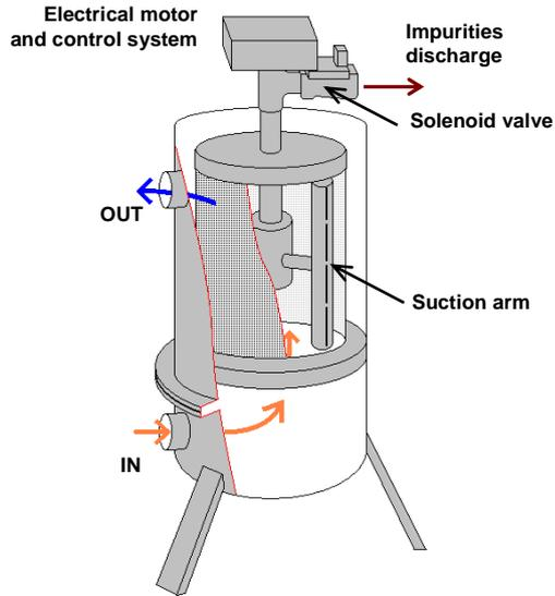
**Filtration.** Filtration is achieved through a multi-layer screen. As soon as the filter screen is clogged, a pressure switch detects the pressure difference between inlet and outlet and starts the cleaning cycle.
