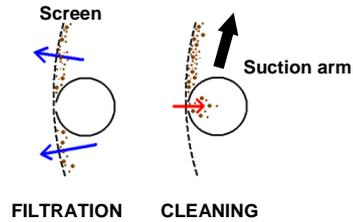
**Drain.** During the cleaning cycle, a solenoid valve is actuated opened and the suspended solids are drained out of the filter.
