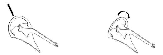
5 - Finally, by placing the pin of the provided shackle (4) through the hole located in the projection of the rear end of the fluke (1), the assembly will be held stably and safely for its use, its uncoupling not being possible without destroying the unit.
