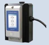
The TW Turb-4 module is a turbidity sensor specifically designed for drinking water applications. With our high measurement accuracy of  $\pm$  (5% + 0.01) and low detection limit of 0.005 FNU, it is possible to detect even the smallest changes in turbidity. Our low detection limit is achieved by our 90° light scattering method. The module is powered by our new power supply, the TW PS300.
