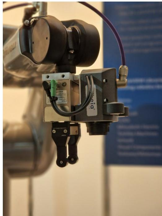
Theia's motorized, NIR corrected IQ Lenses offer the ability to switch between transmitting visible light and Near IR light, enabling high image detail in multi-spectral applications, accurate color rendition in visible light and improved sensitivity in NIR light for a variety of applications including produce inspection and grading, agricultural crop monitoring, Automated Number Plate Reading (ANPR) and many more.
