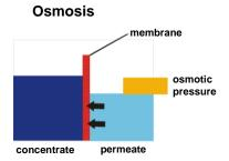
If the sequence is reversed by applying pressure on the higher concentrated solution, clear water penetrates the membrane in reverse direction after the osmotic pressure has been overcome. Dissolved salt is retained. Such process is called reverse osmosis.
