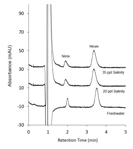
Chromatograms for the analysis of 1 mg  $L^{-1}$   $NO_2^{-}$  and 15 mg  $L^{-1}$   $NO_3^{-}$  freshwater, 20 ppt salinity and 35 ppt salinity sample matrices. Conditions: 120 mM NaCl Eluent, AG15 Column, 235 nm LED Detector
