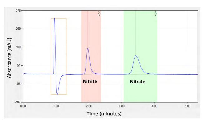
Nitrate: 0.6 - 500 mg/L as  $NO_3^- \mid 0.14 \text{ to } 113 \text{ mg/L}$  as N
