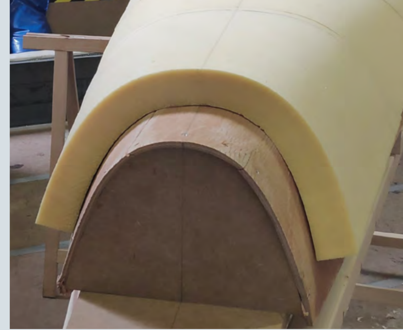
Above: a thermoformed single layer of 40mm Corecell™ M130 for the bow area of a super yacht
