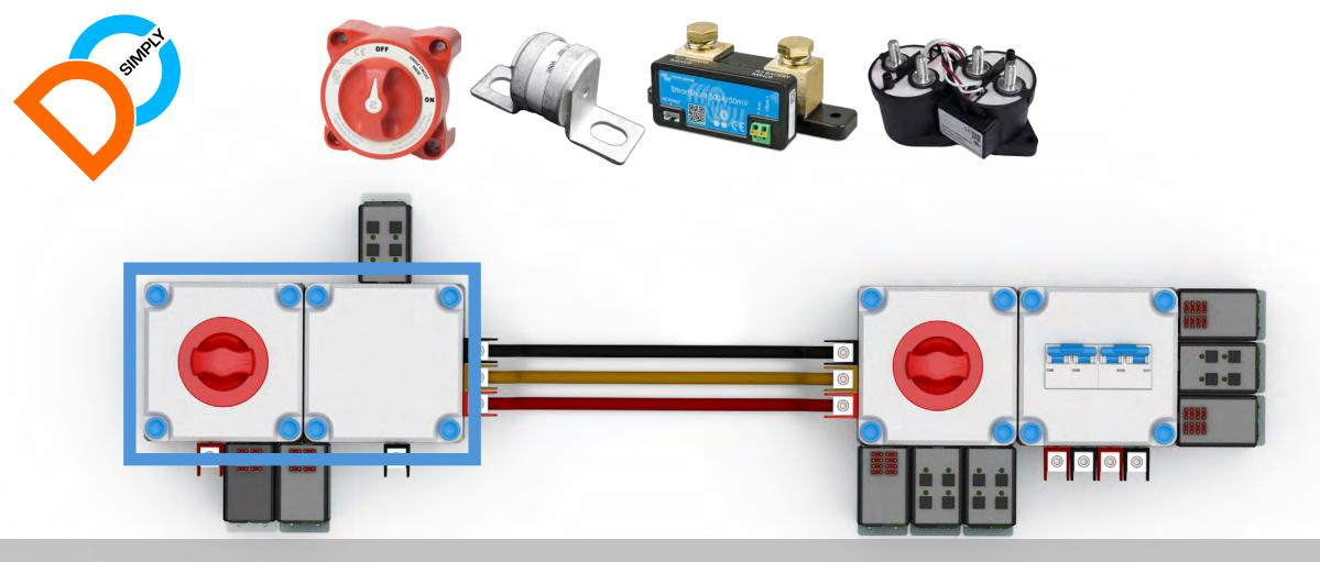
Each Battery bank connected with isolation switch, high current interrupt fuse and optional shunt and contactor (for BMS)
