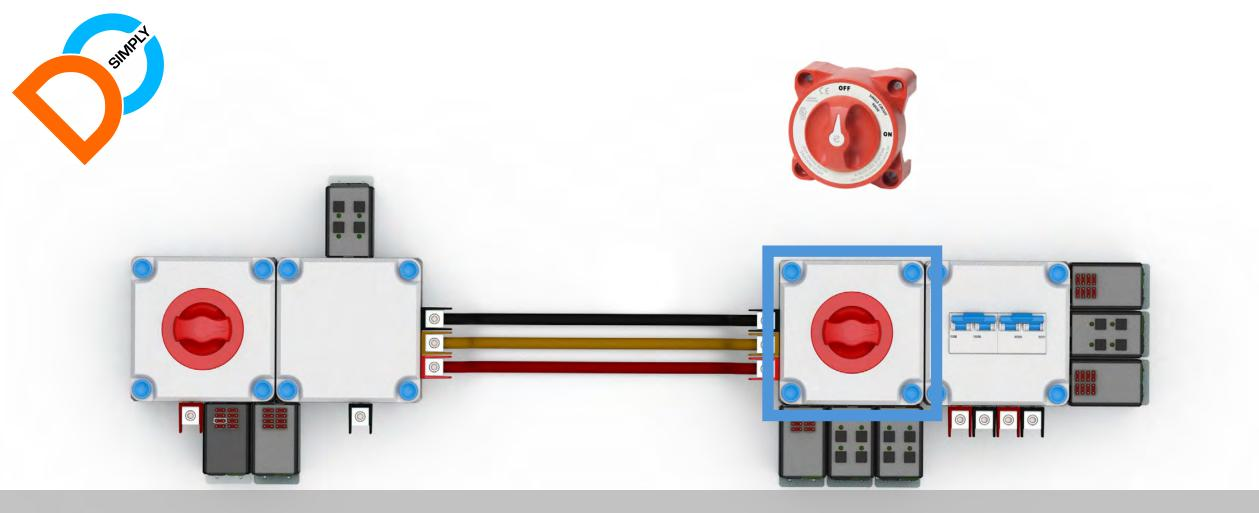
Main switch to switch together the switched on busbar and always on busbar can be located anywhere in the system.
