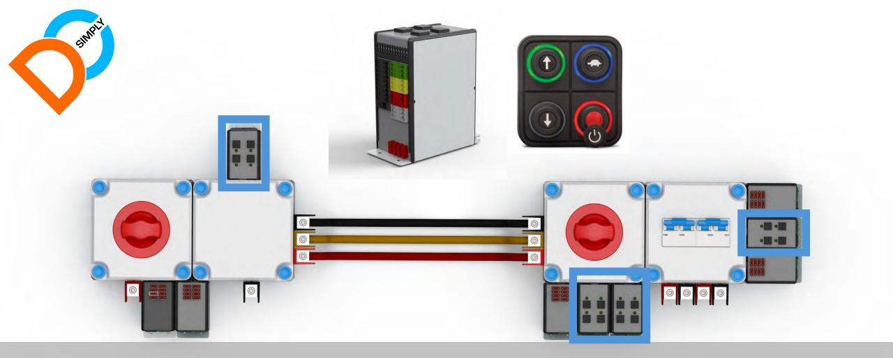
Small 12-24VDC load switching with 4 channel IO Module, with automatic fusing 0,5-8A and optional plug and play 4 button CAN keypad with field insertable icons
