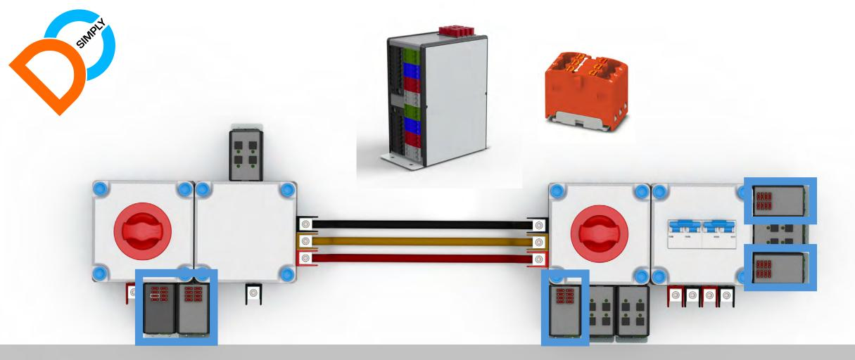
Small DC load connection with 8 channel fused power out module, cable connections with innovative PTFix push in connectors
