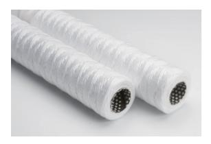
PLX series filter cartridge is made of textile fiber (polypropylene, absorbent cotton or glass fiber) according to a specific process, tightly wound on a porous framework (PP or SS porous tube) to form a honeycomb structure with sparse outside and dense inside, which can effectively filter suspended solids in the fluid, Rust, particles and other impurities, with the characteristics of small pressure drop and large pollutant holding capacity.
