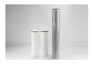
PHF series high flow filter cartridge adopts 6" large diameter (PHFM series is 6.5") structure with single open end. The filter body is divided into two types: PP pleated and melt blown. All connection use thermal welding, no any adhesive, has wide Chemical compatibility, can be applied to food and beverage filtration.
