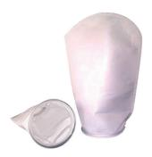
PFB series bag filter is made of needled felt, the filter material has high precision and the surface is treated with singeing, calendering or film coating, without fiber shedding; the thermal welding technology ensures that there will be no side leakage.
