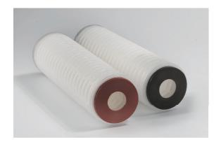
PPM series pleated filter combines the characteristics of depth filtration and pleat technology, ensure high dirt holding capacity and bigger filtration area. It's suitable for filtering high suspended particles, colloidal substances and high viscosity liquids.
