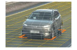
CORE3D unlocks freedom of camera mounting angles, allowing for the camera to capture vehicles accurately even from obliquely-angled viewpoints. This eliminates the requirement of gantry mounting and enables road-side viewpoints of multiple lanes.
