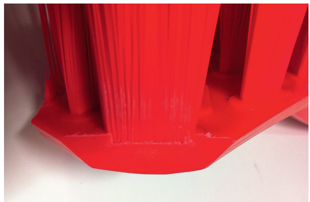
Figure 10d. Vertical cross-section through a UST bristle bundle showing its fully moulded construction.
