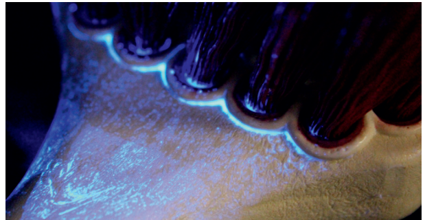
Figure 9a. UV lotion remaining on the fused brush product after brush cleaning.
