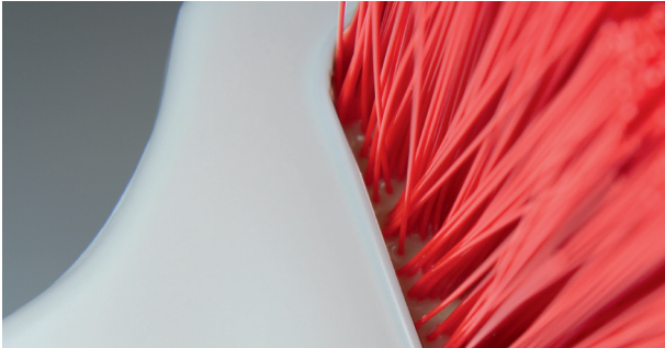
Figure 6a. Resin set brush sample with potential contamination traps.
