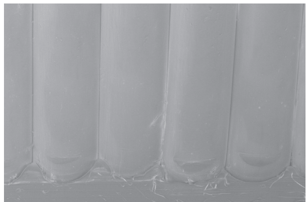
Figure 10c. Scanning electron microscope image of the area where the bristles enter the head of a UST brushware product.
