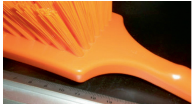
Figure 4a. Drilled and stapled brush sample.
