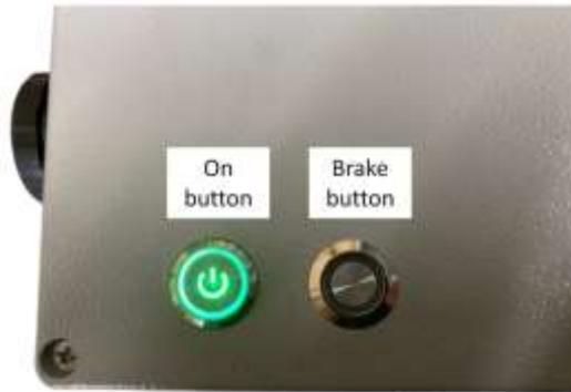
Figure 22: ON button is lit, stop button is not engaged
