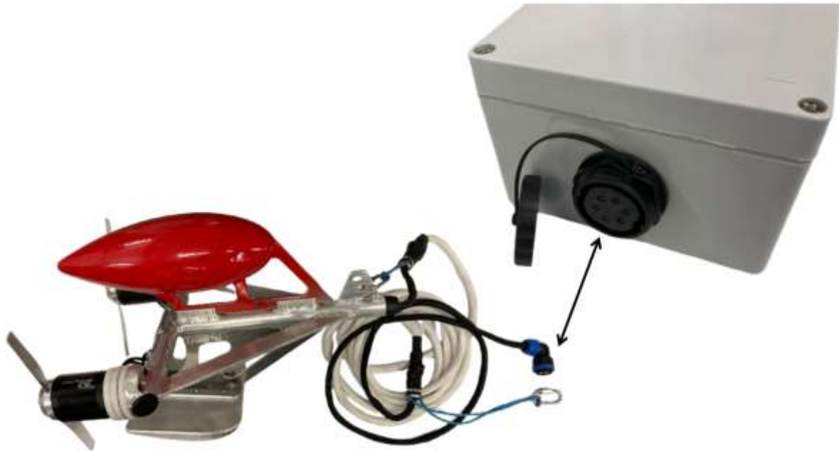
Figure 11: Hydrogenerator directly connected to the electrical box
