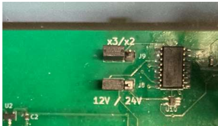
Figure 17: Seawing electronic card and jumpers
