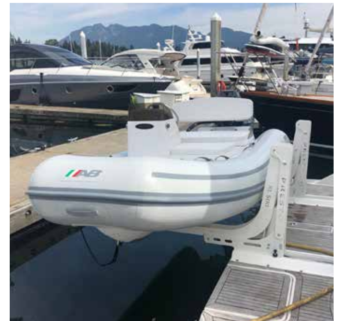
The dinghy safely hangs on the XL500R rail system with a self-adjustable keel support for a rubber boat.
