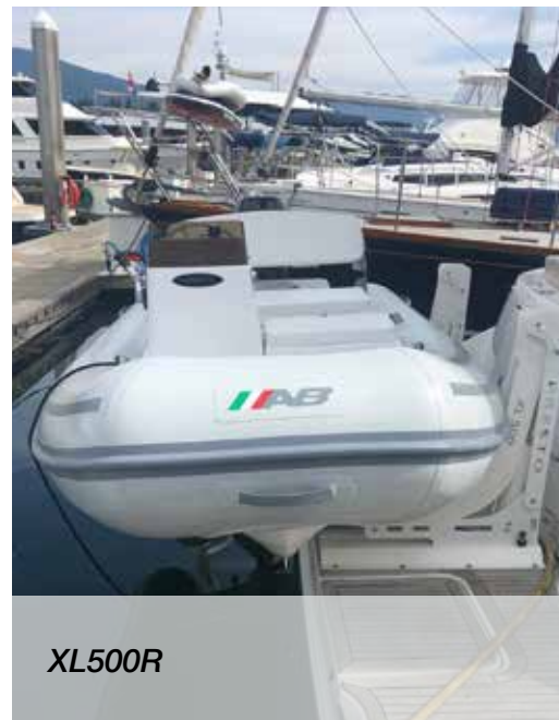
The dinghy safely hangs on the XL500R rail system with a self-adjustable keel support for a rubber boat.
