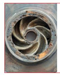
Metallic parts in the seawater fluid path are susceptible to corrosion, erosion, cavitation, and eventual failure.
