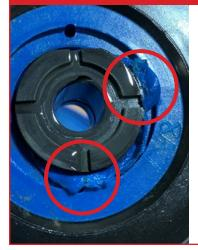
Lower-grade composites are more susceptible to overheating, premature wear, and failure due to friction.
