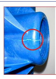
Unreinforced heads crack if excessive force is used or the threads are compromised.
