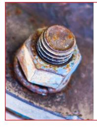
Other pumps use low-grade painted steel hardware that is not made for the marine environment.
