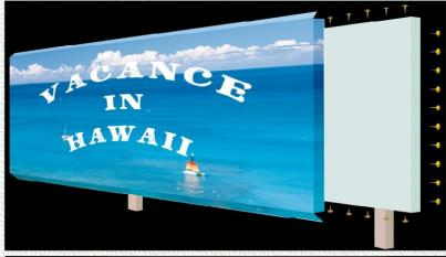
Tarpaulin Fabric can be fixed on the frame with nails, staples or string, as it does not tear easily.
