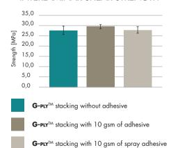
Mechanical performances of the laminate are maintained. Polymerization of the resin is not compromised or inhibited.
