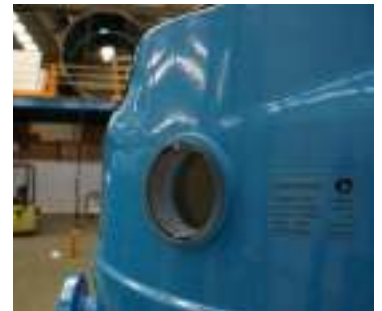
100% full vision inside: Methacrylate sightglasses
