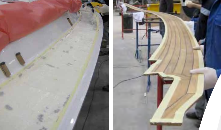
Teak side deck panel being installed with PRO-SET ADV-170/ADV-270
