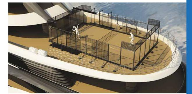
Made from pre-preg carbon fibre, our court components are lightweight but super strong and easy to assemble. We design enclosures for both foredecks and heli-decks with the option of high-strength mesh netting or acrylic panels.
