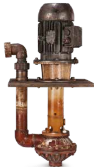
PVDF AS50 PUMP AS50 vertical pump in PVDF for chrome plating bath at a temperature of 80°C. Equipped with elbow fitting designed for system requirements. Length: 465 mm. Maximum flow rate of 40 m 3 /h and maximum head of 25 m w.c.
