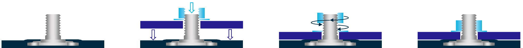
Adjoining component fitted over bigHead stud, retained by nut and washer
