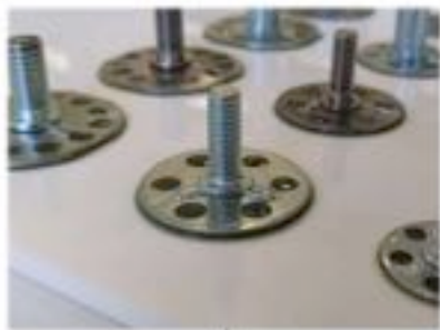
Attachment of bigHeads after the component production (Post-process)
