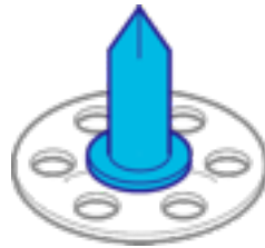
Nail fixing (together with spring clip): Insulation blanket retention
