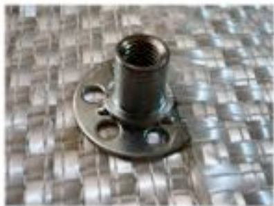
Integration of bigHeads during the component production (Co-process)
